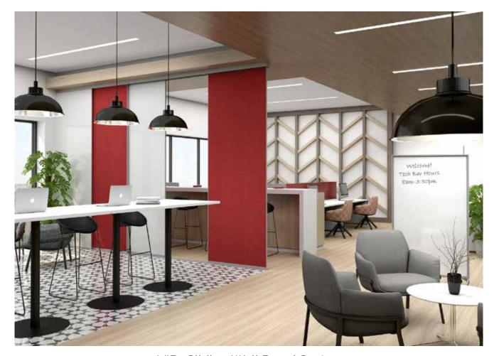
VIP+ Sliding Wall Panel System VIP+ panels make the "in-between" spaces into flexible communication tools. Shown with Triple Track Bottom Rolling, Double-Sided Sliding Porcelain Markerboards and Tackable Fabric Panels.
